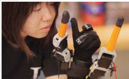
1. Faye Wu, a graduate student in mechanical engineering at MIT, demonstrates the “supernumerary robotic fingers” device. (photo by Melanie Gonick).
