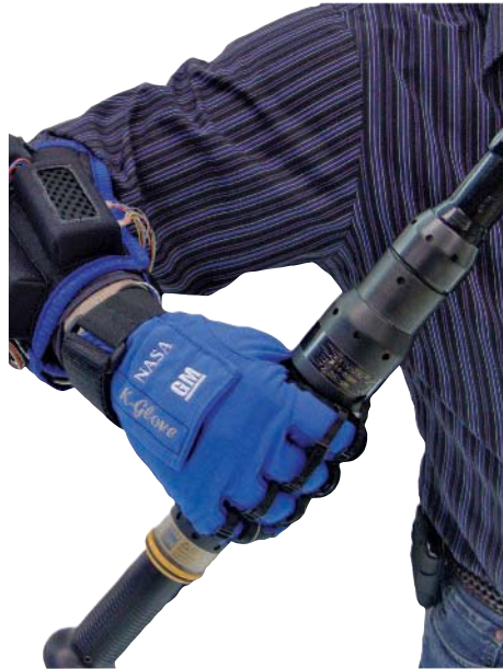
2. RoboGlove is designed to augment a person's grip. It can add force or maintain a grip while the user relaxes.
