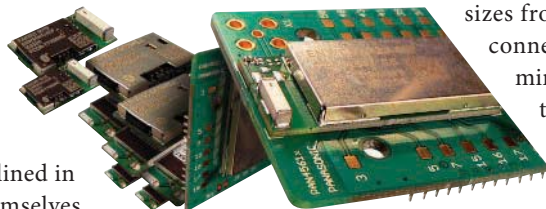
2. Modules based on Bluetooth 4.1 will be able to support more efficient bulk data transfers, greater flexibility in communications between devices, simultaneous dual-mode roles, and the first steps toward IP-based communications.
