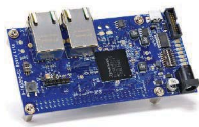
2. The Tessaera R-IN32M3-CL evaluation board includes a pair of RJ45 jacks for EtherCAT support.
