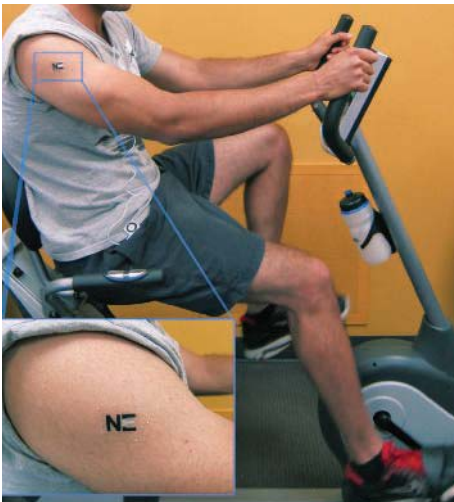
The lactate levels produced during exercise are detected by a tattoo biosensor.
